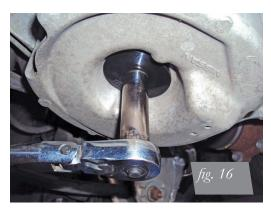
7. Insert the shock assembly into the shock tower and attach the upper bracket to the chassis (fig. 17). Torque the upper bracket nuts to 28 Nm (21 ft-lbs).
