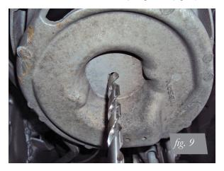
2. To install the nutsert in the upper spring seat, the upper bracket can be used as a template to center the air spring location (fig. 10). Place the bracket against the spring seat and mark the center location. Drill a hole 17/32" (.531" diameter) through the spring seat.
