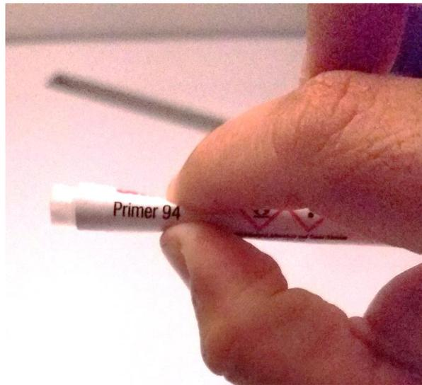
3. Shake the tube back and forth a couple times to get the promoter to flow through the felt tip.
