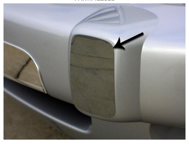
Your new covers come to you with a clear protective liner. Do not remove this liner until installation is complete.
