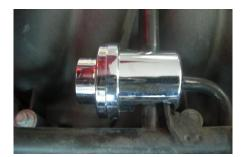
**TECH TIP:** Before placing the end bezel apply a small dab of instant adhesive to the two chrome halves to bond them to each other this will help keep them in place long term. Allow some time for the adhesives to set.
