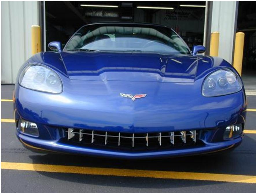
Your new retro grille comes to you preformed however it will be necessary to force the grille into and onto the factory grilles horizontal rib.
