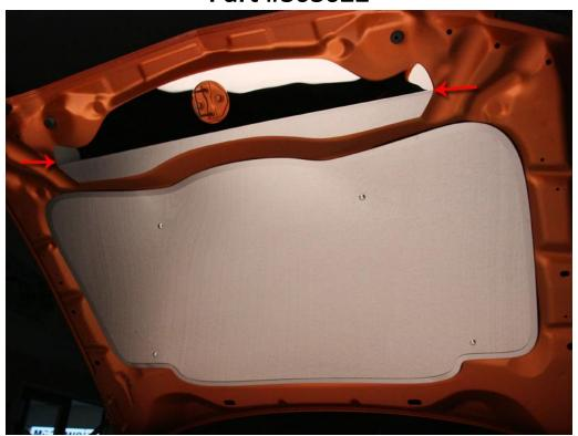
Your cover comes to you with a protective liner. Do not remove liner until final installation.
