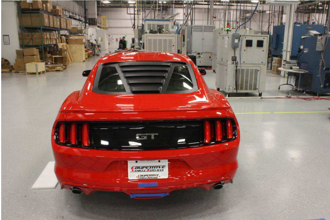
Photograph 22: Rear of Car with Louver
