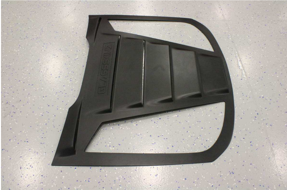
Photograph 20: Rear Louver Sample Side
