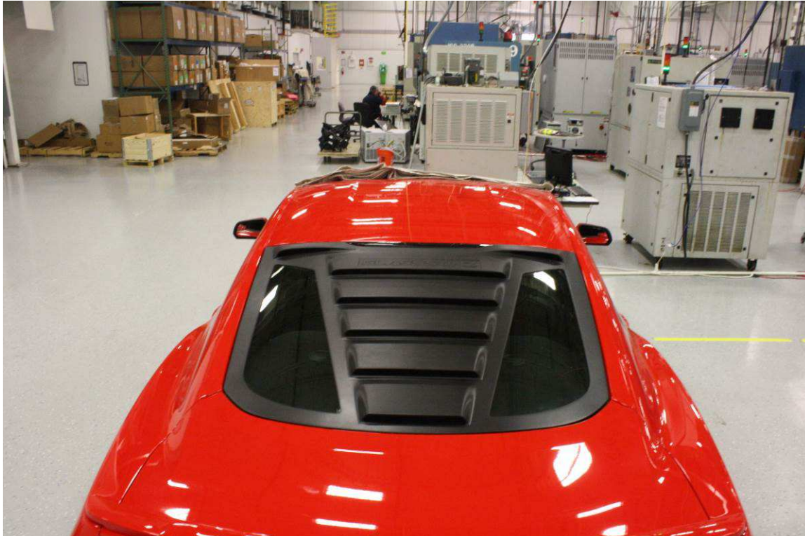
Photograph 14: Louver in Place Overhead
