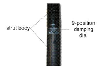
View of Damping Dial on Strut Shaft
